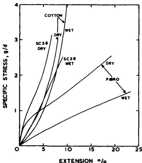
Fig. 7. Load-extension curves for rayon (after Griffiths<sup>11</sup>).
