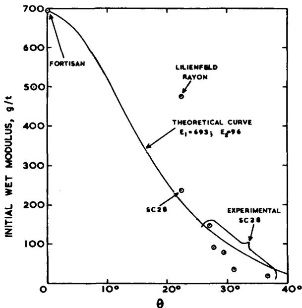
Fig. 6. Variation of modulus of high-modulus rayons with orientation angle; Comparison of experiment and theory (data from Courtaulds<sup>9</sup>).
